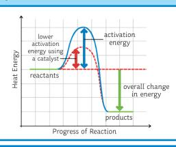
A catalyst is a **substance** that speeds up a chemical reaction without getting used up itself. Catalysts are able to offer an **alternative pathway** at a **lower activation energy**.
